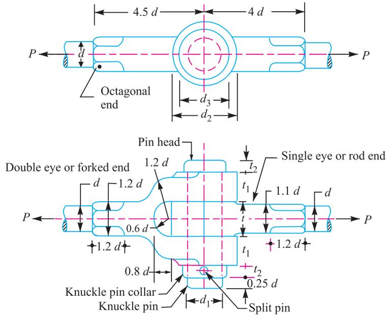
Fig. 12.16. Knuckle joint.
