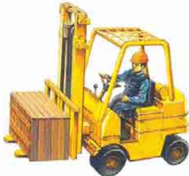
Fork lift is used to move goods from one place to the other within the factory.
