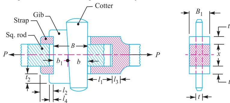
**Fig. 12.13.** Gib and cotter joint for square rods.
