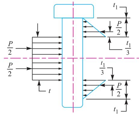
Fig. 12.17. Distribution of load on the pin.
